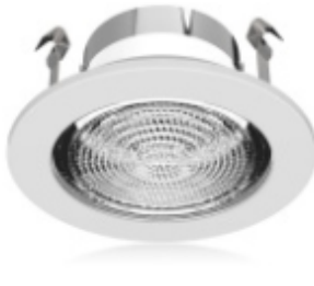
TSL-62 1/4 Inch Shower Reflector Trim with Fresnel Lens Lamp: R20/PAR20 35W max Gasket used to prevent moisture Wet location listed
